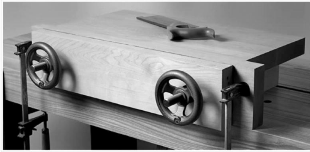
A previous version of our Moxon handwheel on a benchtop bench.
