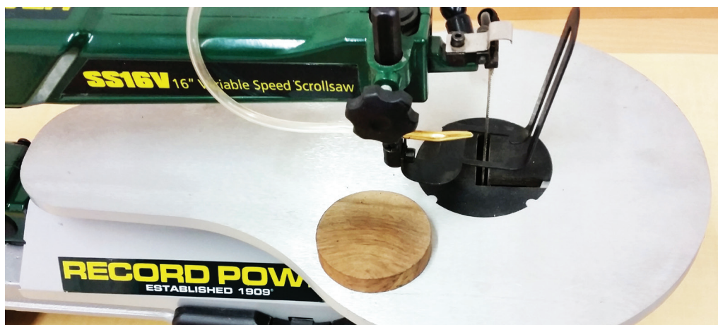
Photo 2: Cutting a circular blank on a scrollsaw
