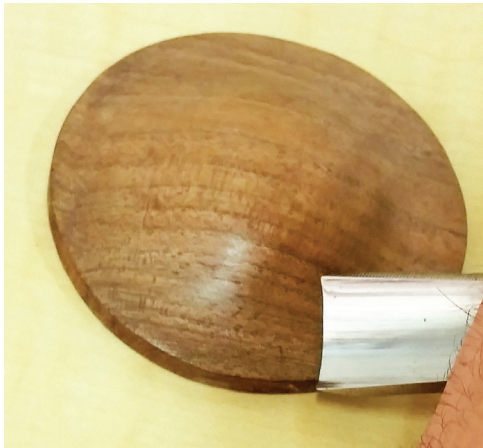
Photo.4: Thinning the edges with tool #12
