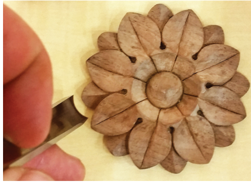
Photo.11: Shaping the tips of the small petals.
