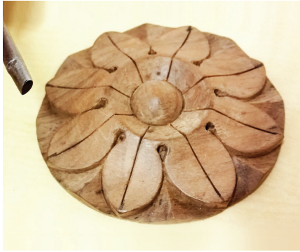
Photo.9: Using a home made punch to refine the teardrop shape at the base of each petal.
