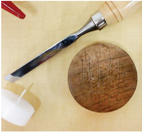
Photo.3: Gluing the blank to a board after scoring the back and applying some candle wax.
