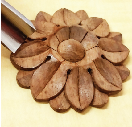
Photo.10: Forming the V-shape in each large petal.
