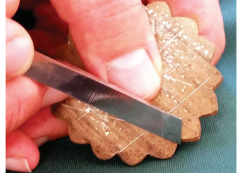
Photo.14: Reducing the back of the tips to a fine point with chisel #1
