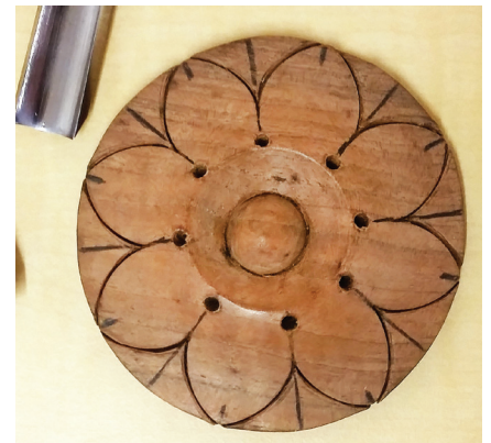
Photo.7: Rounding over the centre button and outlining the petals.
